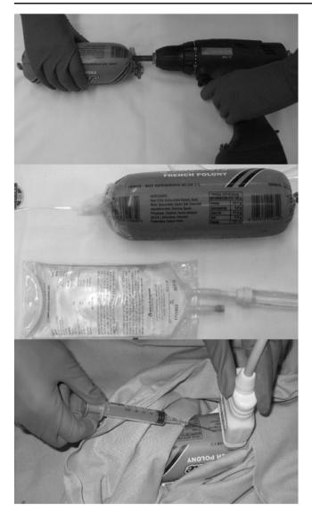
Fig. 1 The construction of the central venous access polony phantom. First a hole is carefully bored from one end of the polony with a lowspeed drill, then an expired IV is connected to keep the vein filled. Standard techniques can be used for the simulated vascular access
